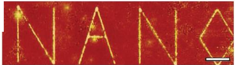
Fig. 1. Optical superlensing experiment. The embedded objects are inscribed onto the 50-nm-thick chrome (Cr); at left is an array of 60-nm-wide slots of 120 nm pitch, separated from the 35-nm-thick silver film by a 40-nm PMMA spacer layer. The image of the object is recorded by the photoresist on the other side of the silver superlens.
