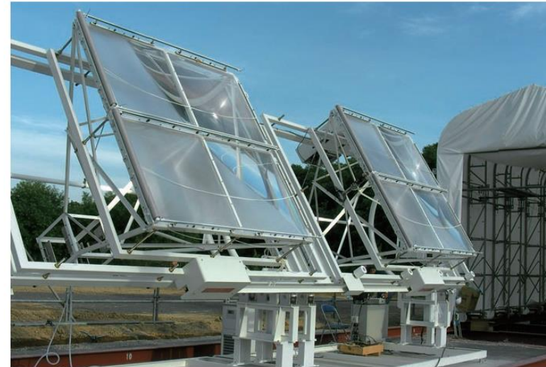
Figure 2 A schematic of the solar-powered laser design. A high-performance 1.3-m 2 Fresnel lens collects the light and a highly efficient, broad-absorption-band chromium-doped Nd:YAG ceramic laser gain medium enables most of the Sun's wide spectrum to be captured.
