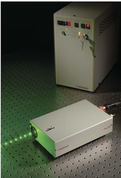
The Minilite platforms offer users accessible harmonic generators, integrated energy attenuator and simple operation. Both the Minilite I and II lasers, use a single YAG rod/flashlamp pump chamber, invar resonator, and a stable resonator design which offers maximum energy extraction and excellent beam quality.
